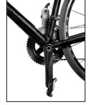
6. If the zeroing has not worked successfully, you will observe the numbers 999 or -999. This indicates that the arms are not sufficiently vertical or stable. Adjust the position to vertical or steady the bike and try again. If the calibration fails again, change the battery. In the unlikely event that re-zeroing continues to fail, please contact support@4iiii.com for further assistance.
