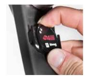
Use the battery cap tabs to twist the cap into the unlocked position (rotate left).
