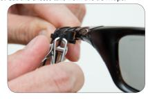
**7.** Slide your Sportiiiis unit back onto the mount, bend the boom into its final position.
