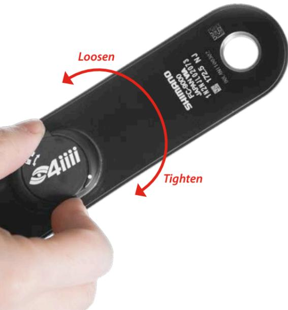
1. Do not pry your battery cap. To remove, twist the battery cap counterclockwise on your powermeter
