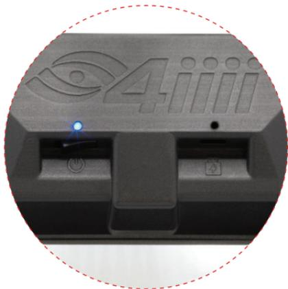
**Warning:** For safety reasons, do not charge the trainer below 5°C (41°F). Doing so may result in damage to the lithium ion battery, explosion, or injury.
